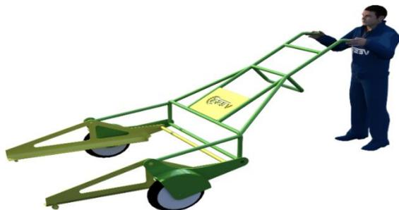
**DEUX PALETTES PAR BROUETTE DE TRANSPORT MANUEL :** APRES LA REALISATION DE LA PRESSE, LES PRODUITS FINIS SONT TRANSPORTES AU SECHAGE VIA CETTE BROUETTE. SA CONCEPTION ERGONOMIQUE FACILITE SA MANIABILITE AU TRANSPORTEUR. POUR UN MOUVEMENT EN SERIE NOUS AVONS CHOSI DES PNEUS A AIR. AVEC LES PNEUS A AIR, LES TRANSPORTEURS FERONT TOUS TYPES DE MOUVEMENT AVEC FACILITE. ELLE EST CONÇU POUR TRANSPORTER DEUX PALETTES PLEINES.
